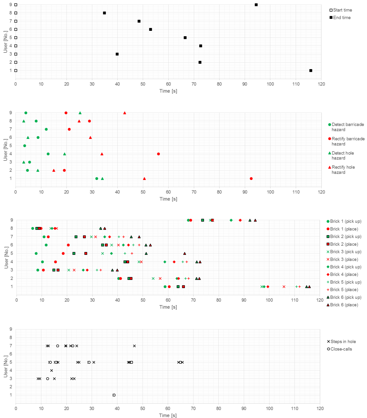
Fig. 8: Analysis of synthetic data (timestamps) recorded of users in VR, from top to bottom: Start/end time of user experience, detection/rectification of two hazards (leading edge and floor opening), picking/placing masonry bricks as work task, and steps-in/close-calls in floor openings.
